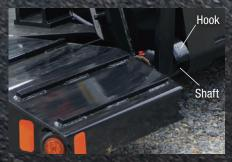
Hydraulic removable "shaft & hook" gooseneck is the fastest and most versatile in the industry—especially on uneven ground.
